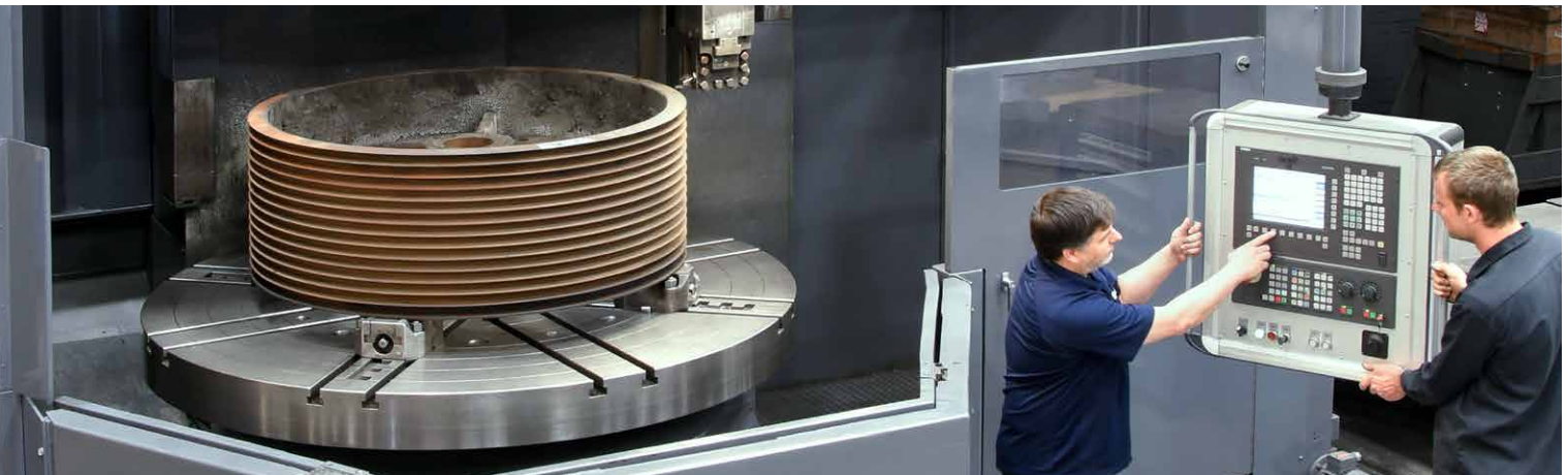
TOS VTL vertical turning lathe for machining mid- to large-sized workpieces
